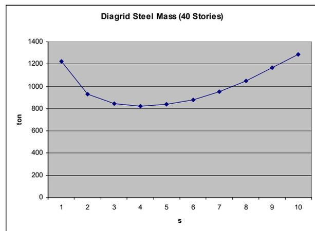
Figure 15: 40 Story Diagrid Steel Mass
